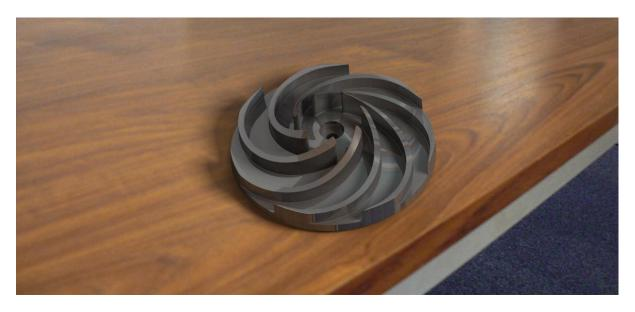
Heart pumps need precision impellers optimised for high RPM, flow rate and multi-decade longevity. This design is a scaled-up prototype impeller optimised to run at 2700RPM across a 0.8 bar pressure difference and achieve a 75 litres/min flow rate.
