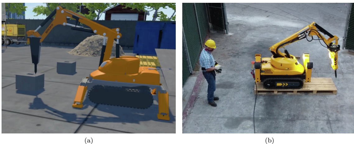
Figure 6: VR-based simulation for training demolition robot operators. (a) Demolition robot in simulated construction environment. (b) Real demolition robot being operated. [35]
