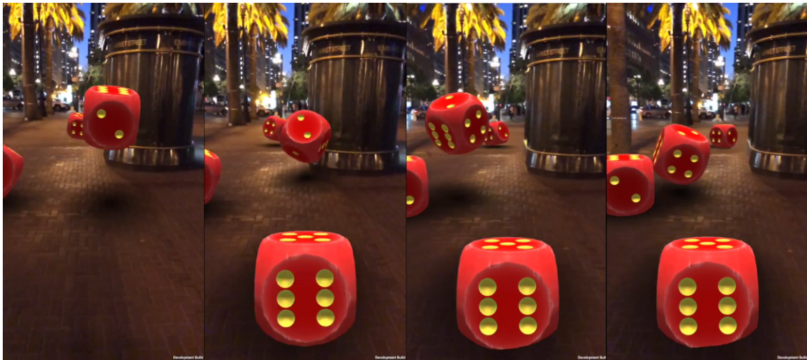
Figure 7: Niantic’s Lightship ARDK provides mobile developers with an easy to implement AR-physics solution using PhysX as its backbone, here virtual die are thrown producing basic elastic collisions with surfaces in the real world [40]
