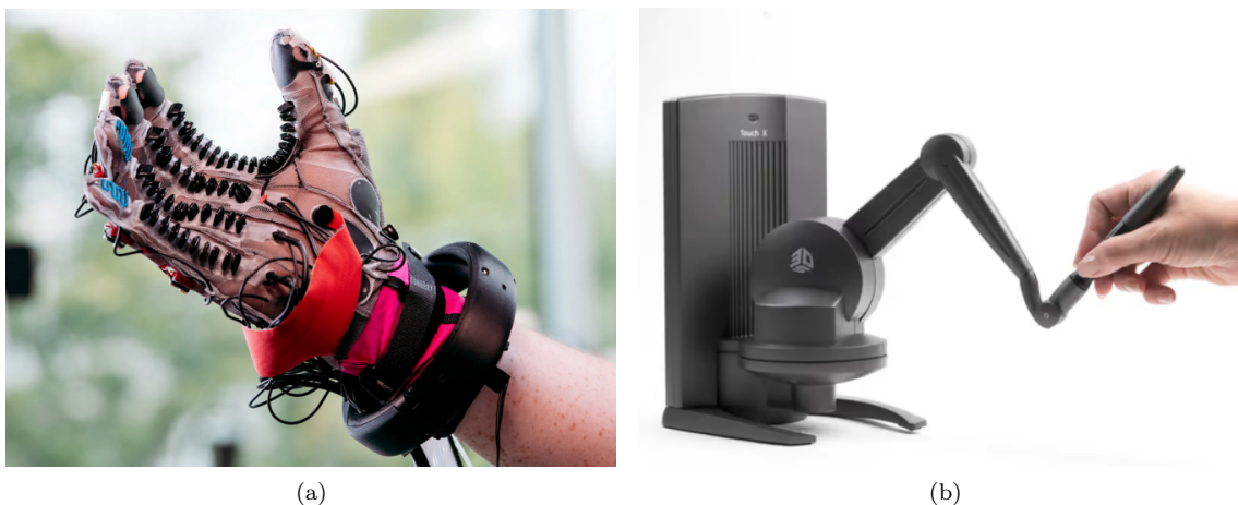
Figure 5: Examples of haptic devices. (a) Meta’s early stage haptic glove. (b) TouchX haptic device by 3D Systems. [30, 31]
