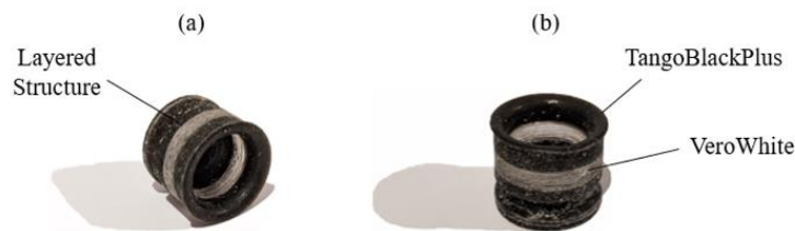
Figure 22: Early version of self-sealing suction cup. (a) Side view. (b) Front view showing TangoBlackPlus and VeroWhite material used to create flexible and rigid layers.
